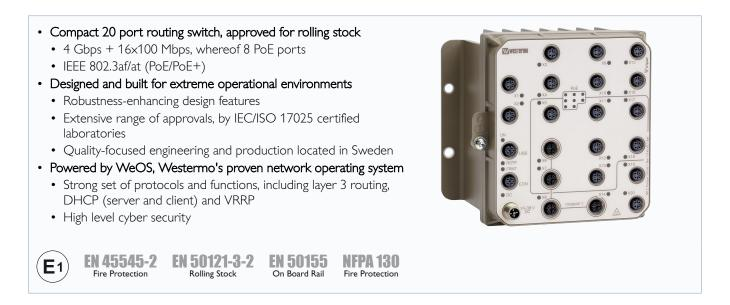
The Viper-220A-T4G-P8-LV is a managed 20 port routing switch optimised for the needs of the railway rolling stock market. PoE ports offer effective powering of end-devices. Gbps ports cope with high bandwidth devices such as access points and NVRs (Network Video Recorders).
