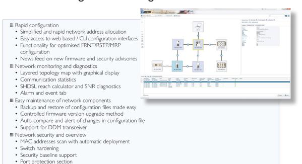
WeConfig is a Network Configuration Management (NCM) tool that simplifies both the installation of a data communications network and the ongoing maintenance after commissioning has been completed. WeConfig scans the network for devices and displays discovered units and their connections on a topology map. Basic IP address configuration, as well as global parameter settings, can be quickly assigned and further configuration easily facilitated.
