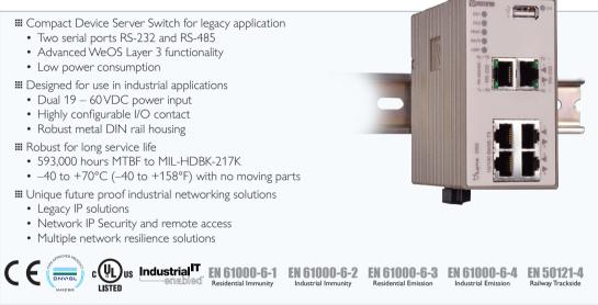
Lynx DSS is available in several versions, the L206-S2 is a device server with a layer 3 industrial Ethernet switch, powered by the Westermo WeOS network operating system. Lynx DSS is the most compact and has the lowest power requirements in this class of device servers. Lynx DSS has 4 10/100 Mbit/s ports and two serial ports. One of the serial ports is configured for RS-232 the other one can be configured for RS-232 or RS-422/485.
