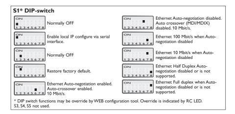
Note! DIP-switch alterations are only effective after a power on.
