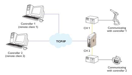
It is also possible to direct the two serial servers to the same serial channel, useful for redundant SCADA.
