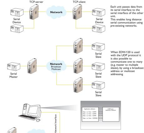
EDW-120 can also provide a remote serial interface for a computer connected through a TCP/IP network using a Virtual IP software.
