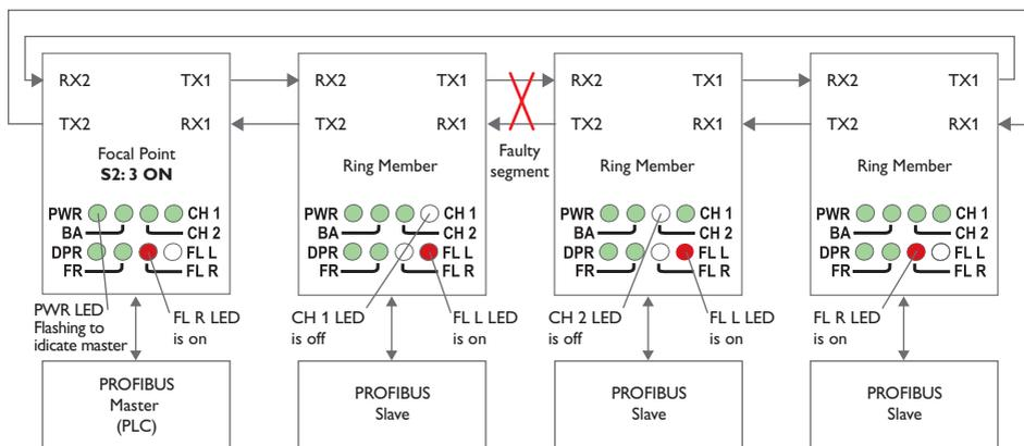
If an optical fibre segment fails, the ODW-710-F2 focal point will switch mode and start sending out data on both optical fibre ports, CH 1 and CH 2, simultaneously.
