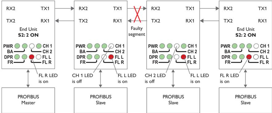
If an optical fibre segment fails, all communication with units beyond the faulty fibre segment will be lost. To determine which fibre segment has failed, look at the FL L, CH 1 and CH 2 LED's as show in the picture above.
