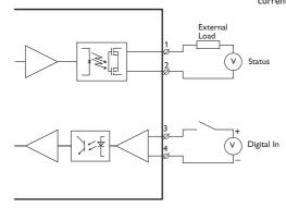
The Digital in is an opto-isolated digital input which can be used to monitor external events. For voltage/current ratings, see Interface Specification section:
