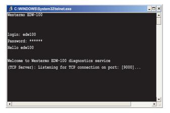
The Telnet diagnostic service provide the user with information such as UDP- or TCP mode, connected or listening state (TCP) etc.
