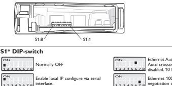
Ethernet Auto-negotiation disabled. Auto crossover (MDI/MDIX) disabled. 10 Mbit/s. Ethernet 100 Mbit/s when Autonegotiation disabled 2345 ON Ethernet 10 Mbit/s when Auto-Normally OFF negotiation disabled Ethernet Full duplex when Auto-ON negotiation disabled or is not Restore factory default. 8 2 3456 7 supported. Ethernet Half Duplex Auto-ON Ethernet Auto-negotiation enabled. negotiation disabled or is not Auto-crossover enabled. 2 3 4 5 6 7 8 supported.
