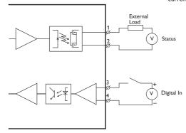
The Digital in is an opto-isolated digital input which can be used to monitor external events. For voltage/current ratings, see Interface Specification section:
