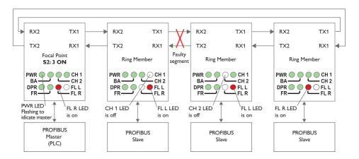
If an optical fibre segment fails, the ODW-710-F2 focal point will switch mode and start sending out data on both optical fibre ports, CH 1 and CH 2, simultaneously.
