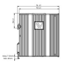
**Dimension W x H x D**  $52 \times 100 \times 101 \text{ mm}$
