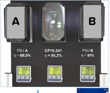
Figure 1: Experimental setup after a 4-hour runtime
