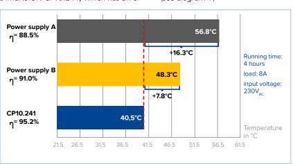
Illustration 1: The effects of efficiency on waste heat in the 240W device class
