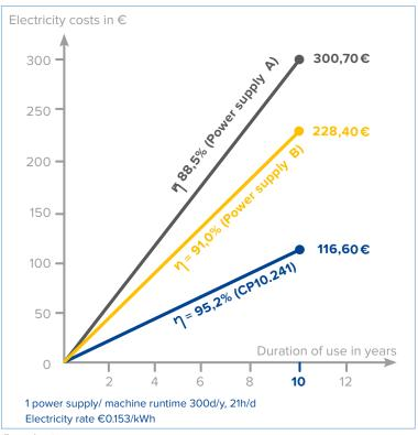
Illustration 2: The effects of efficiency on electricity costs in the 240W device class
