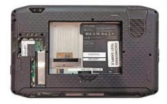
Opening the R12 is a bit of a challenge because several of the small Philips head screws that hold the two halves of the tablet together are hidden underneath little rubber plugs, some of which blend into the housing's dotted surface treatment pattern. Once all have been found and undone, the two halves separate.
