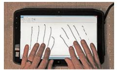
For a very long time, tablets used either resistive touch that worked with a finger or a passive stylus, or they had an active digitizer with a special pen, usually of the Wacom variety, and sometimes they used both together. That all changed when first the iPhone and then the iPad popularized capacitive multi-touch with its effortless panning and pinching and zooming.
