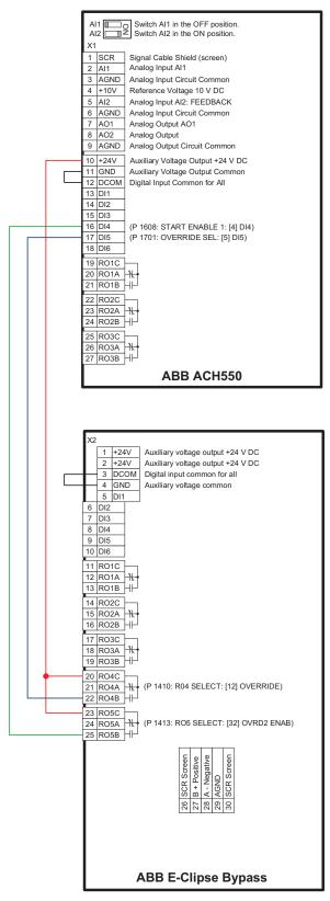
Recommended control wiring between ACH550 and E-Clipse Bypass to enable Advanced Override 2.
