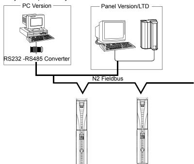
On the N2 Fieldbus each system can be accessed by the full complement of Metasys FMS features, including Change-of-State (COS) monitoring, alarm notification, scheduling, trend, and totalization.
