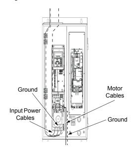
Power connections – Standard E-Clipse Bypass configurations (wall mounted)
