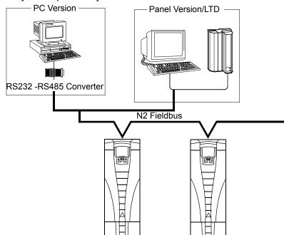
The following diagram shows the drives' integration to the Johnson Controls Metasys Companion system.
