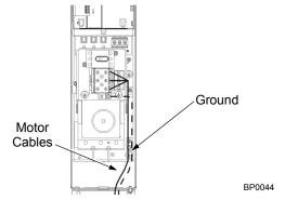
Motor connections – Standard E-Clipse Bypass configurations (wall mounted)
