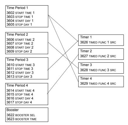
A parameter can be connected to only one timer.
