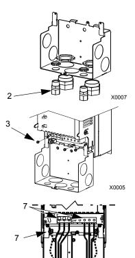
**Note:** For R5 frame size, the minimum power cable size is 25 mm<sup>2</sup> (4 AWG). For R6 frame size, refer to *Power terminal considerations – R6 Frame size* on page *1-307*.
