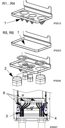
**Note:** For R5 frame size, the minimum power cable size is 25 mm<sup>2</sup> (4 AWG). For R6 frame size, refer to *Power terminal considerations – R6 Frame size* on page 1-307.
