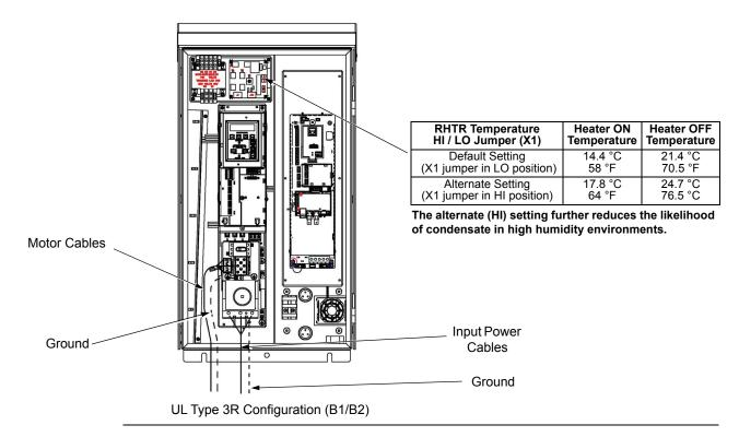
**Note:** UL Type 3R, B1/B2 enclosures are designed to be mounted on a wall. Mounting these 3R enclosures on an open rack system requires the use of the supplied 3R enclosure back plates to maintain 3R integrity.
