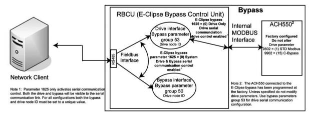
Figure 1 - Communications physical and logical connections
