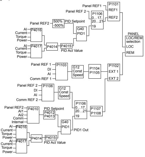
**Note:** In order to activate and use the PID controller, parameter 1106 must be set to value 19.
