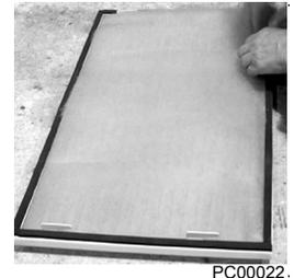
7. Reinstall the filter restrainers.
