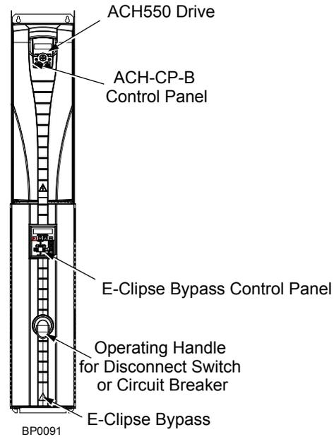
The following shows the front view of the ACH550 E-Clipse Bypass standard configurations, and identifies the major components.
