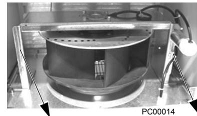
5. Disconnect the fan wiring and capacitor from the fan frame. Then remove the four screws attaching the fan to the fan frame. Remove the old fan.
