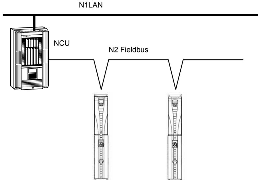
The following diagram shows the drives' integration to the Johnson Controls Metasys Companion system.
