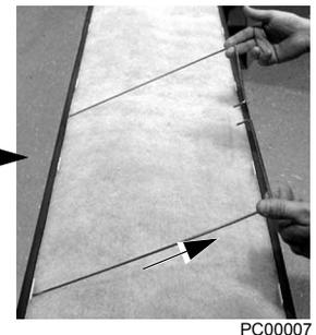
3. Install the replacement filter. Be sure to tuck the filter into the groove around the entire filter frame. This is very important for proper installation.
