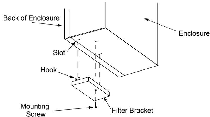
3. Lift the filter out of the filter bracket and replace as appropriate.
