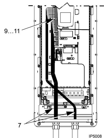
*R7...R8, wiring (both enclosure types)*
