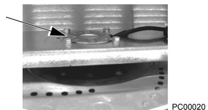
6. Install the new fan and capacitor with the replacement part for ABB in the reverse order of the above. Ensure the fan is centered on the velocity stack and rotates freely.
