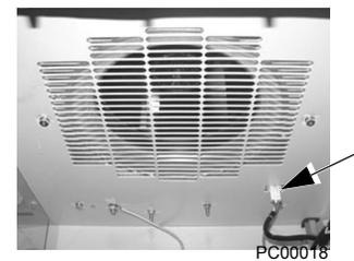
3. Undo the four fastening screws at the corners of the fan frame. The screws are through bolts with nuts on the inside of the cabinet. (Do not drop the hardware into the drive).
