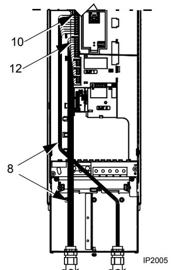
*R1...R6, wiring UL type 12 enclosure*
