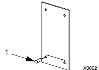
**Note:** Frame sizes R3 and R4 have four holes along the top. Use only two. If possible, use the two outside holes (to allow room to remove the fan for maintenance).
