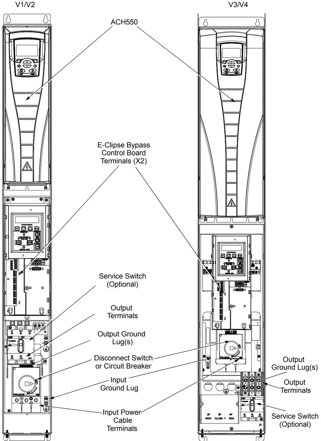
Connection diagrams – Standard E-Cclipse Bypass (wall mounted)
