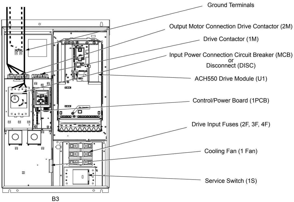
*Connection diagrams – Standard E-Cclipse Bypass (R8, floor mounted)*
