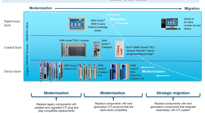
\* CTI 2500 Series CPUs are 100% compatible with TI/Simatic 505 CPUs in all applications except for those using the XSUB instruction
