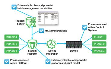
This platform integration simplifies building a common real time data model across all manufacturing operations which may span across receiving, batching, filling, packaging and shipping. InBatch execution information is available to be directly leveraged by other software functionality such as Wonderware Historian or by Wonderware MES Software.
