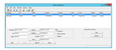
The batch scheduling function maintains a list of batches to be produced. The user can opt to select any listed batch for execution unless the system has been configured to enforce batch execution in order.
