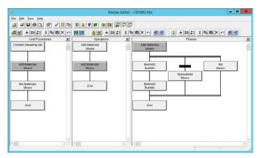
The InBatch Recipe Editor uses the information in the process model and materials management as part of recipe procedure development. An InBatch master recipe may or may not be size specific and can be assigned to any process line that fits the equipment requirements defined in the recipe. All formula quantities for ingredients, intermediates, by-products and finished goods are configured as either actual quantities or scalable as a percent of the batch size.
