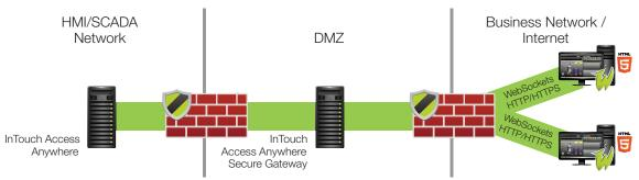
No data is transferred, only mouse clicks, keystrokes and gestures from the remote user to the RDP host and graphics from the RDP host to the client end
