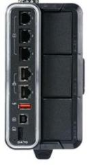
DA70 3 Comm. Sleds 3 Serial Ports 2 Ethernet Ports USB Host USB Device
