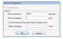
Setting the failover expression to true, for example by setting the failover tag to true, switches the Access Name from the primary (false) to secondary (true) I/O data sources.
