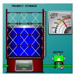
The analog meter symbol you embedded in the Reactor window shows the same tank volume value as the digital read-out at the bottom of the tank.
