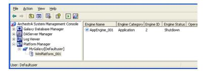
3 In the details pane, locate the engine and view its status in the **Engine Status** column.
