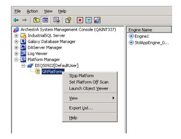
When you start Object Viewer from Platform Manager with a platform or engine selected, the utility starts and shows the attributes of the selected platform or engine. After Object Viewer is launched, it becomes independent from Platform Manager.
