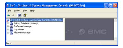
The left pane, or console tree has a Windows Explorer-type layout, with the ArchestrA System Management Console appearing as the root node and the Platform Manager appearing below this node. You can expand and collapse the console tree by clicking on the "+" or the "-" symbols that appear next to the snap-in.
