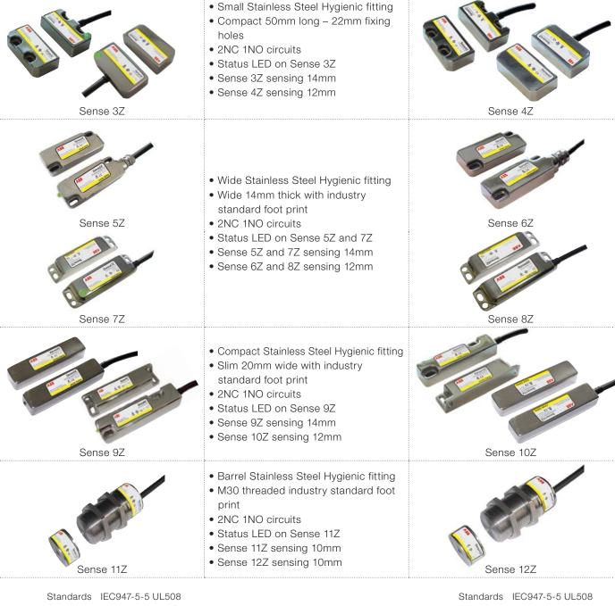
Enclosures Stainless Steel 316 Protection IP69K / IP67 Sensing 10-14mm typical Ambient Temp. -25C, 80C Mechanical Life 3,300,000 operations Operational Rating 24V 200mA Contacts 2NC/1NO StandardsIEC947-5-5 UL508EnclosuresStainless Steel 316ProtectionIP69K / IP67Sensing10-12mm typicalAmbient Temp.-25C, 105CMechanical Life3,300,000 operationsOperational Rating240V 1AContacts2NC/1NO
