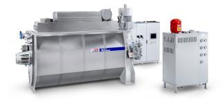
A mid-sized line processing 2-3 tons of chocolate per hour is made up of a couple of refiners and 4-5 conches, with total installed power exceeding 1 MW.
