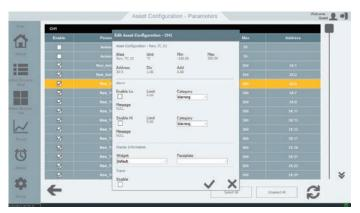
**OPC:** InTouch Edge HMI provides native OPC interfaces, such as OPC UA (Client/Server), OPC DA (Client/Server), OPC XML (Client), OPC .NET (Client), and OPC HDA (Server). OPC UA and OPC DA also offers native redundancy configuration.
