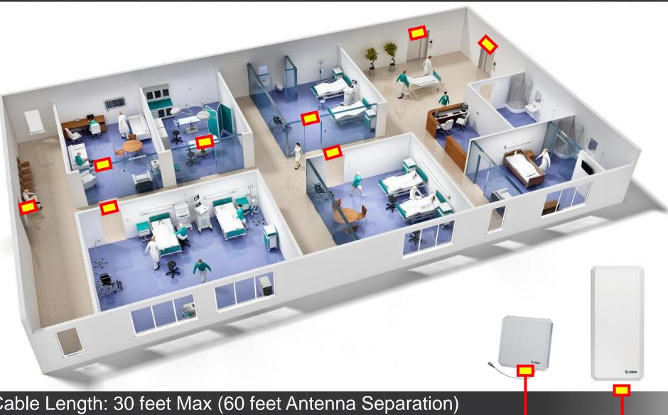
Antenna Cable Length: 30 feet Max (60 feet Antenna Separation)
