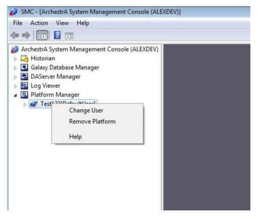
Please remember to use this supported method. Platform Killer shouldn't be used for System Platform 2012 and above. Platform Killer can created problems requiring a system to be reformatted on 2012 and above. Even for versions before 2012 it is better to try the supported method first then try Platform Killer.
