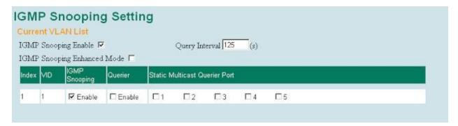
Firmware in both switches is the same. Both will forward EIP traffic. Both can be accessed via an Allen Bradley ControlLogix add-on instruction. The part number difference is only to enable IGMP snooping by default. The non-EIP switch can be configured to be a -EIP switch by making the configuration change above. Note: one switch in the network must be enabled as the Querier.
