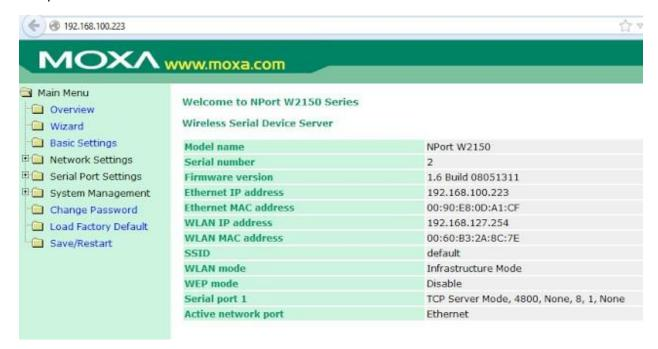
Out of the box, this unit has a default IP address listed on the back. It features a built-in web server for configuring the IP address and serial port baud rate.
