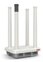
The TropOS 1420 provides superior reliability by accessing 653 MHz of RF spectrum (463 MHz in ETSI) using automatic interference avoidance capabilities of TropOS Mesh OS. It uses the 802.11a/b/g/n wireless standards to deliver 600 Mbps total wireless data rate, 300 Mbps at 2.4 GHz and another 300 Mbps at 5 GHz.
