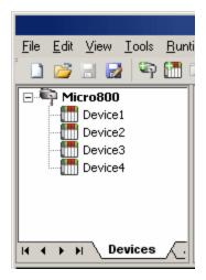
Each device appears under a single channel, called "Micro800". In this configuration, the driver must move from one device to the next as quickly as possible in order to gather information at an effective rate. As more devices are added or more information is requested from a single device, the overall update rate begins to suffer.
