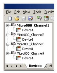
Each device has now been defined under its own channel. In this new configuration, a single path of execution is dedicated to the task of gathering data from each device. If the application has 256 or fewer devices, it can be optimized exactly how it is shown here.
