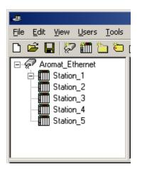
Each device appears under a single Aromat Ethernet channel. In this configuration, the driver must move from one device to the next as quickly as possible in order to gather information at an effective rate. As more devices are added or more information is requested from a single device, the overall update rate begins to suffer.
