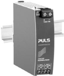
The YR40.242 is equipped with two input channels, which are individually decoupled by utilizing mosfet technology. Using mosfets instead of diodes reduces the heat generation and the voltage drop between input and output. The YR40.242 does not require an additional auxiliary voltage and is self-powered even in case of a short circuit across the output.
