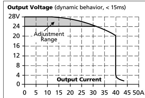
Fig. 6-3 **Short-circuit on output, Hiccup<sup>PLUS</sup> mode, preliminary, typ.**
