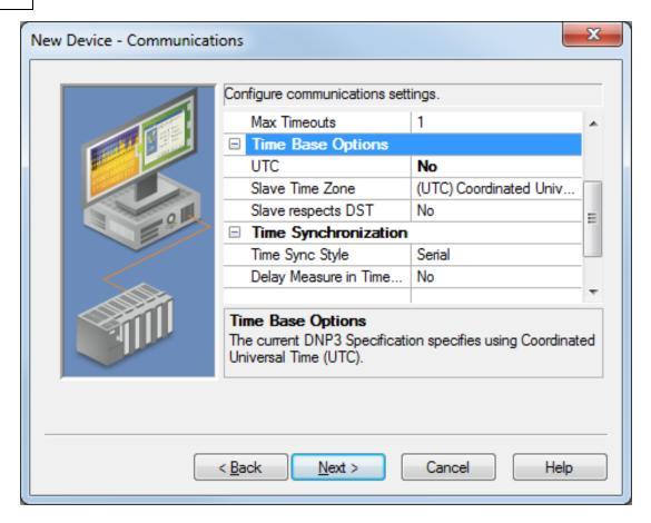
• **UTC:** This parameter specifies the time base of the DNP slave to be used during time synchronization and event time of occurrences. When Yes is selected, Universal Coordinated Time is used. The default setting is Yes.
