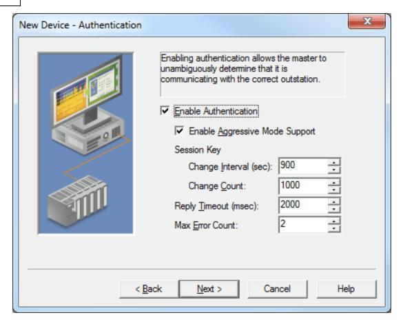
• **Enable Authentication:** When checked, this parameter enables authentication. If the device requires authentication, the master must configure it as well. The default setting is unchecked.
