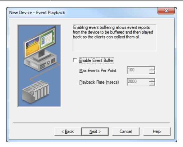
• **Enable Event Buffer:** When checked, this option allows event reports from the remote DNP device to be buffered and played back for OPC client collection. The default setting is unchecked.
