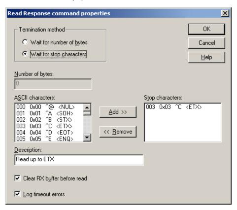
5. Once the response has been received and copied into the read buffer, commands must be added to parse the data and send the result to the appropriate tag. The <u>Update Tag</u> command does just that. There must be an Update Tag command for each tag in the block. For Tag\_1, users know the data starts at byte 2 in the read buffer. The device data format defined for Tag\_1 tells the driver to parse up to the next comma. The command properties for Tag\_1 will look as shown below.
