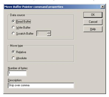
9. If users expected values to be separated by a comma space, then they would have entered 2 in **Number of bytes**. Now the read buffer pointer points to the first byte of value 2. The Update Tag command for Tag\_2 should appear as shown below.
